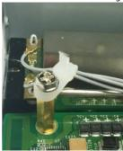
18. Plug the antenna onto the connector.
